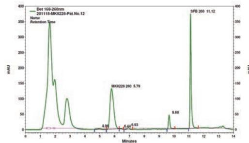
HPLC run of the determination of letermovir (MK8228, concentration 4.731 ng/ml). SFB = sorafenib = internal standard.
