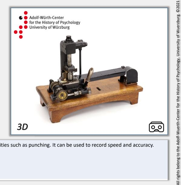
This test was developed to check work performance in monotonous activities such as punching. It can be used to record speed and accuracy. It was mainly used in the transport sector in France.
