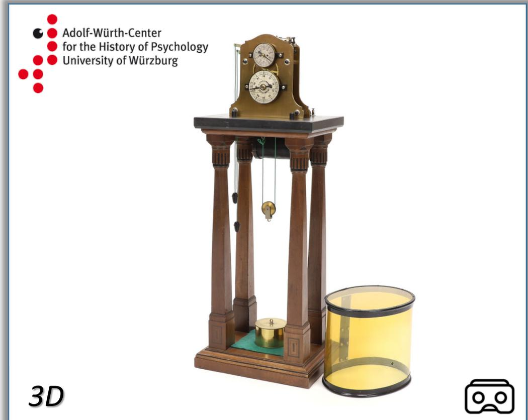
By decoupling the clockwork and the hands using an electromagnetic mechanism, Matthäus Hipp improved the chronoscope around 1848, making it possible to measure time in the millisecond range. At the beginning of the 20th century, Rudolf Schulze succeeded in further developing Hipp's construction by using polarized magnets instead of electromagnets, which he patented (DRP 209 151).
