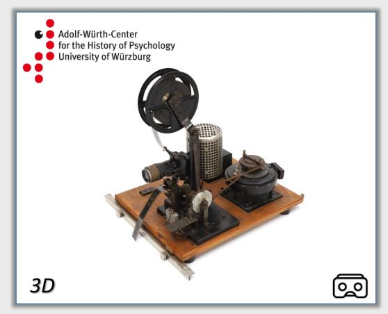
This apparatus for continuous exposure essentially consists of a film projector which can either be operated picture by picture by the test person via a magnetic switch or which advances at equal picture intervals via a contact metronome. On the film, arithmetic tasks for measuring the mental performance of the test person are shown. Not shown is an opal glass pane with a viewing window of 13 by 18 centimeters, which is fixed to a metal bar in front of the projector with two screws.
