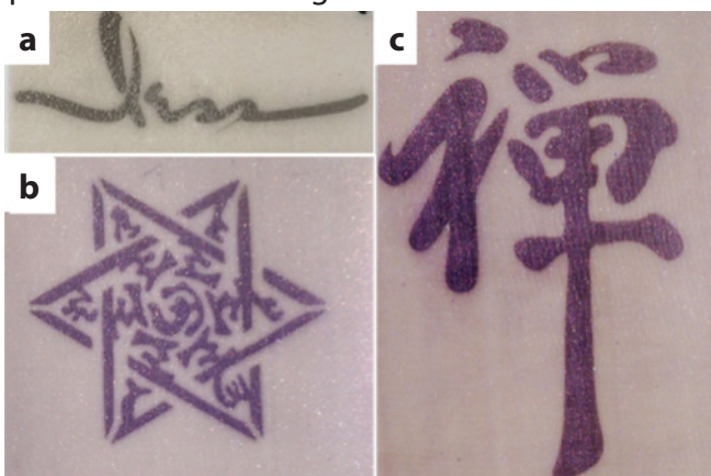
FIGURE 5 ❖ a) Signature, b) pattern, c) Chinese character radiated into photosensitive coating.
