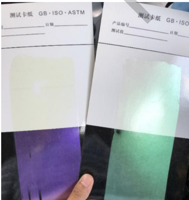
FIGURE 3 ❖ Iridescent coatings show different color on top of a white or black base.
