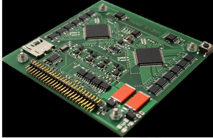
**Fig. 3:** UWE-3 on-board data handling system with two redundant low-power consumption microcontroller units
