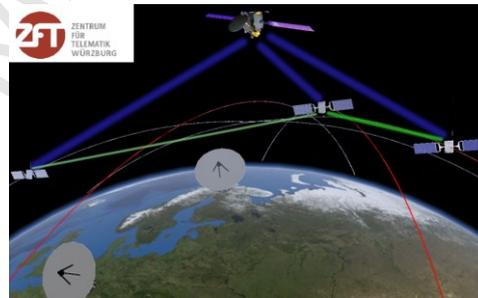
**Fig. 4:** Typical Network of cooperating multiple satellites and ground stations
