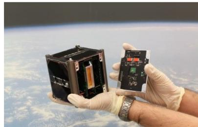
**Fig. 1:** The pico-satellite UWE-3 providing a fully functional spacecraft at 1 kg mass.
