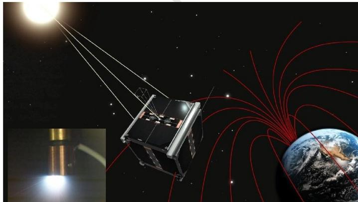
**Fig. 5:** The planned in-orbit demonstration of attitude and orbit control by UWE-4 based on an electric propulsion system (lower left corner during laboratory tests). Sun sensors and magnetometers are used for attitude determination, as well as magnetorquers and reaction wheels for attitude control.
