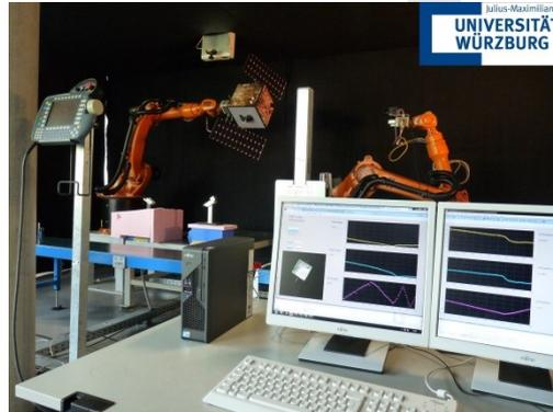
**Fig. 6:** Simulation of dynamics in rendezvous & docking by robots with a passive satellite (mounted at left side) to determine position and attitude from servicer sensors (mounted at right side).
