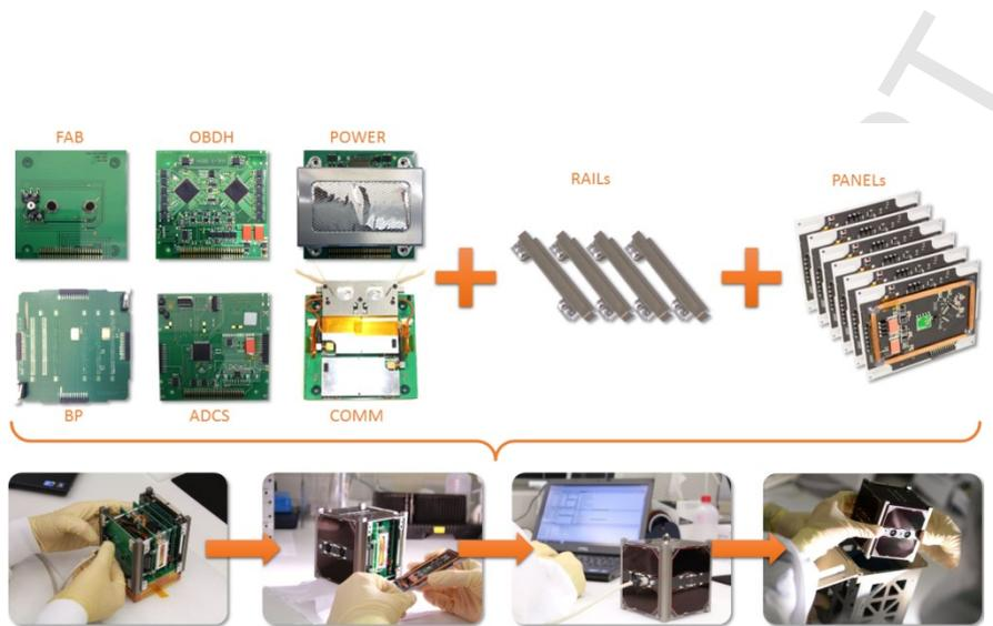
**Fig. 2:** Integration of subsystems and satellite components taking advantage of flexible modular design architecture
