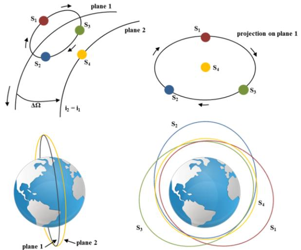
Figure 4: NetSat-4G Cartwheel-Helix formation (orbits not to scale) [17].
