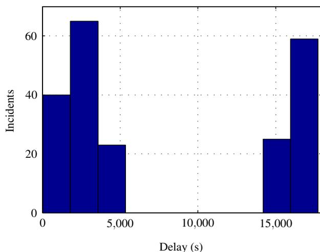
**Fig. 7** Message (bundle) delay histogram (distribution) for a message delay of 30 s
