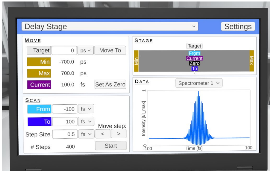
Figure 14. Automatic scan carried out with the delay stage UI. The scan parameters (From, To, and Step Size) can be entered in the Scan panel (bottom left) and the scan can be started by Start. Acquired data is plotted in the Data panel. In the present example, an interferometric autocorrelation received from integrating the second harmonic of the output of a Michelson-type interferometer was measured (bottom right).
