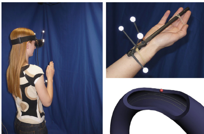
Fig. 8. Rest position (left), hand tracking body fixation (top right) and steam tube object with particle flow (bottom right).
